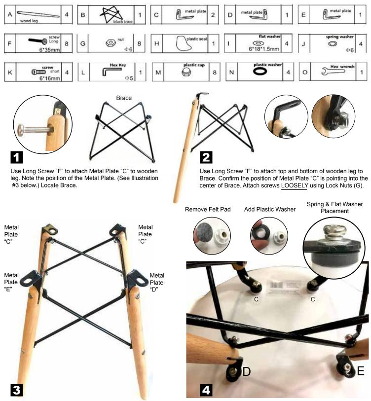
Use Long Screw "F" to attach remaining legs and Metal Plates "C", "D", and "E" in the position as shown above using long screw and lock nuts. Note the position of the Metal Plates "D" & "E" are pointed out. (See Illustration #3.)
