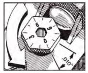
**G.** Always file depth gauges so filing stroke is from the inside of the cutter to the outside.
