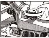
**D.** Move cutter backwards until file is directly above the depth gauge.
