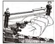
C. Mount file guide assembly on the guide bar so that the chain guide T-bars (5) are flush with the top of the chain rivets. Tighten assembly with locking thumb screw (8).
