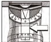
**C.** Turn adjusting screw (12) and lower file until it rests on the top plate of the cutter.
