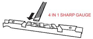
File all cutters on one side. Move to other side of chain and file all cutters opposite to complete sharpening. File all cutter identically.
