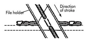
• If damage is present on the chrome surface of top plates or side plates, file back until such damage is removed.
