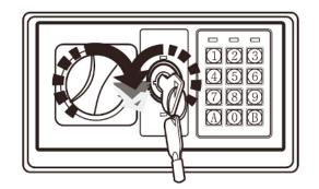
This lock requires (4) AA batteries (1.5V). Under normal use, batteries will last about 1 year. When the battery is low and you press a button on the keypad, a red warning light indicates the battery is low.
