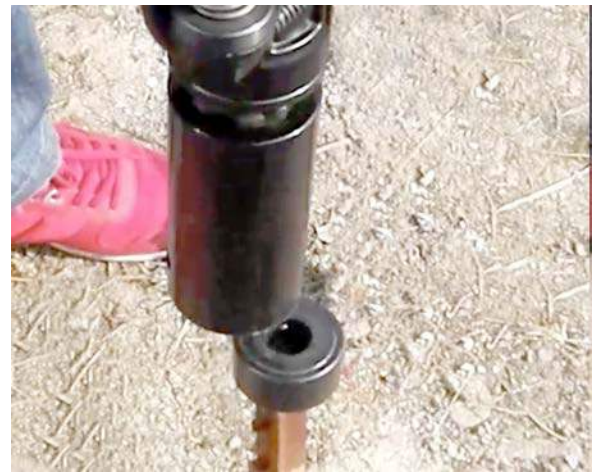
Fig. 4 ) Insert Inner Pile Head \Phi 67 . Use a wood handle or metal bar to force inside Sleeve.
