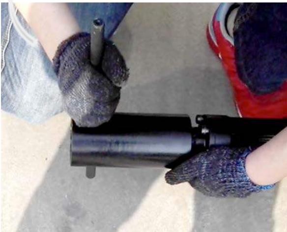
Fig. 3 ) Insert Socket Pin, then rotate Piling Socket Sleeve to make sure it is tight & secure.
