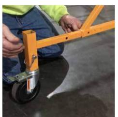
Choose one of the nine settings, then use the Connector Pins (BB) to lock the outrigger in place.
