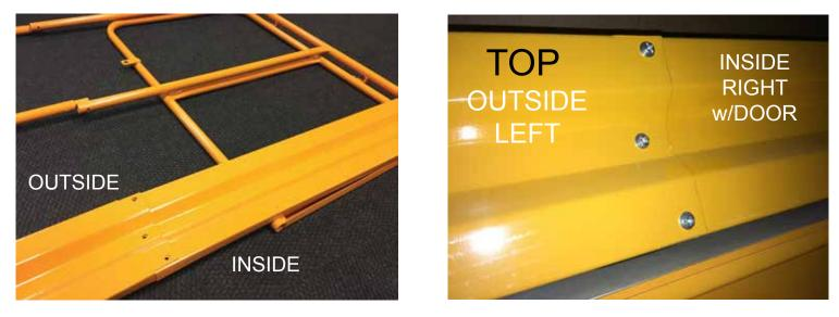
6) Position Guard Rails On Top of Scaffold, Insert Into SQUARE Frame.
