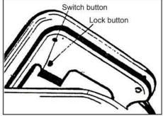
2. Locate the Power Trigger (Switch Button) and Lock Button. Use the Lock Button to provide locking to the ON/OFF power button.
