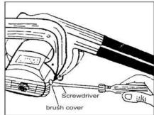
3. Over time, the carbon brush may need to be replaced. Follow the diagram above to locate and replace the brush.
