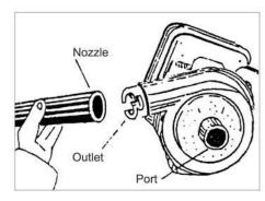
1. Attach the Nozzle to the Outlet. This will provide the necessary angle to the blower.
