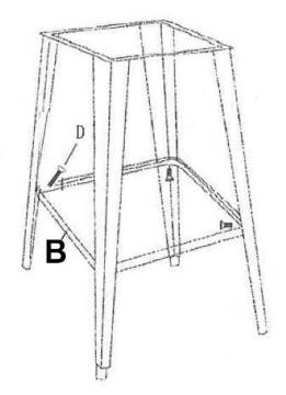
2. Attach Leg Support (B) to each Table Leg (C) using 4 screws (D).
