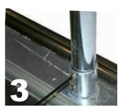
Using the hex wrench, loosely tighten the hex set screws (with the HEX side visible) into the corner support.
