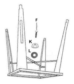
4. Attach X-support (B) using 1 piece screw (F), washer (L) and nut (K).
