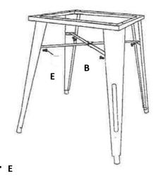
3. Attach 1 piece X-support(B) using 4 pieces small screws (E).
