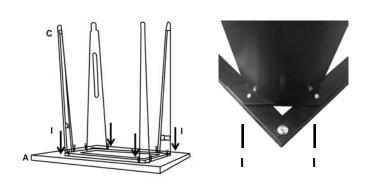
2. Attach each Table Leg (D) to Table Top Frame (C) using 8 pieces medium screws (1).
