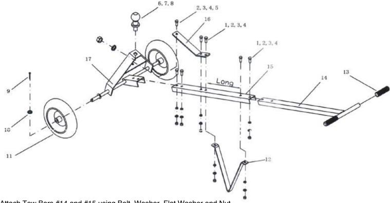
Attach Tow Bars #14 and #15 using Bolt, Washer, Flat Washer and Nut.
