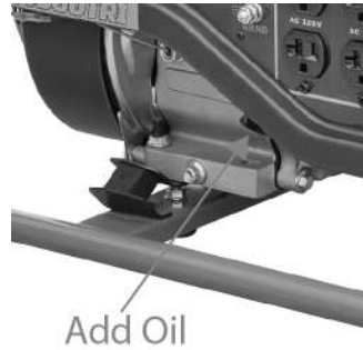
Figure 11 - Checking the Oil
