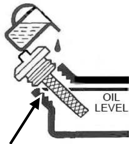
Figure 2 - Add Oil To TOP Of Threads
