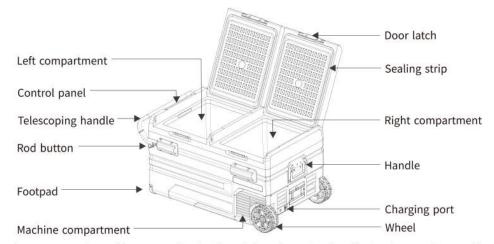
\*Note: press the rod buttons on both sides of the telescoping handle simultaneously to pull the rod.
