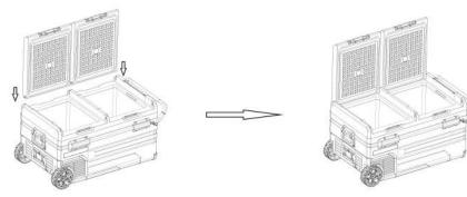
Align the door shaft with the compartment hole and insert it
