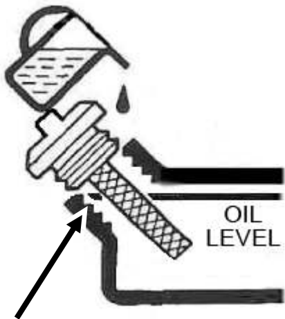
Figure 2 - Add Oil To TOP Of Threads
