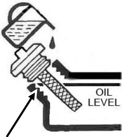
Figure 2 - Add Oil To TOP Of Threads
